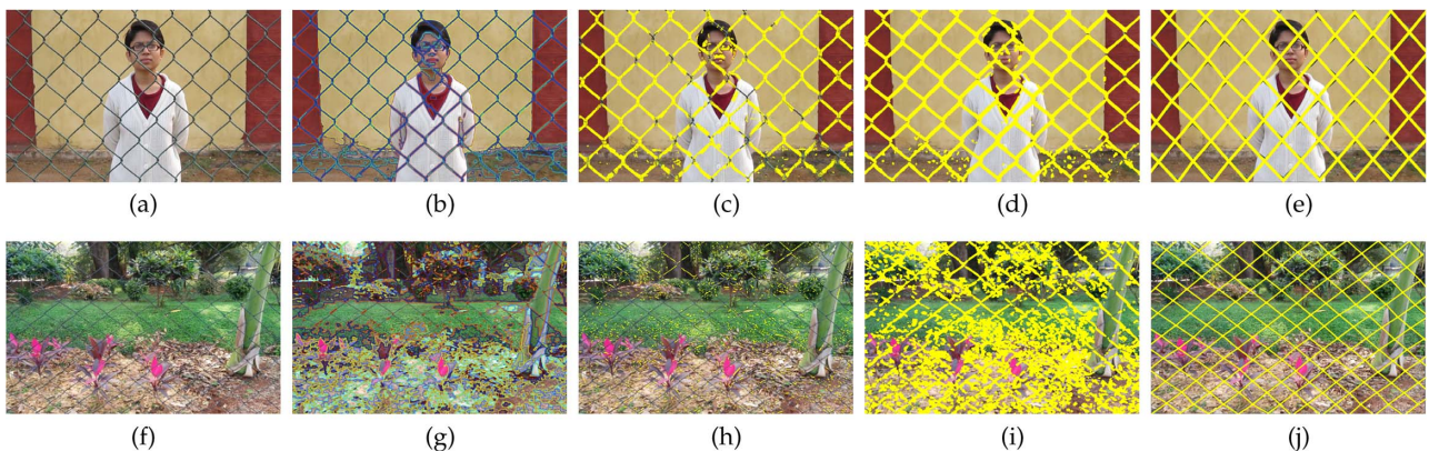
Fig. 3. (a), (f) Two observations chosen from two videos of fenced scenes. (b), (g) Segmentation results obtained using [36] for (a) and (f), respectively. (c), (h) Detected fence pixels using SWT [40]. (d), (i) Estimated fence masks using Gabor filter [41] responses obtained for (a) and (f), respectively. (e), (j) Fence masks obtained for observations (a) and (f) using the proposed algorithm.
