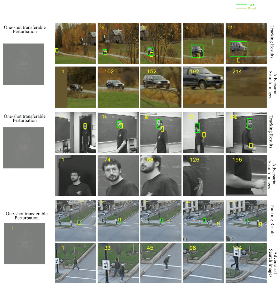
Figure 6.8 – Qualitative results for untargeted attacks with our approach (Ours) on the SiameseRPN++(M) [144] tracker with \epsilon = 16 . We visualize the tracking outputs, the adversarial search regions and the single temporally transferable directional perturbation computed from the object template. Green represents the ground-truth bounding box, and yellow represents the predicted bounding box. We observe that the perturbation is concentrated around the center region and effective to fool the tracker for the entire video sequence.
