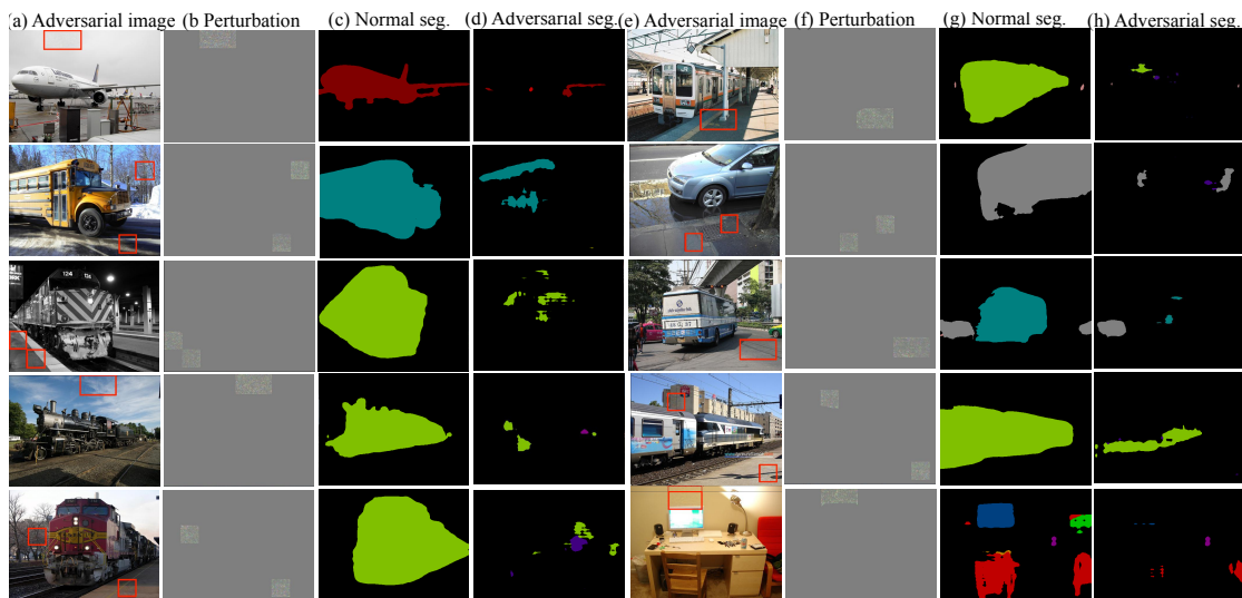
Figure 5.4 – Adaptive indirect local attacks on PASCAL VOC with PSANet [311]. An adversarial input image (a),(e) when attacked at positions shown as red boxes with a perturbation (b),(f) is misclassified within the foreground object areas of the normal segmentation map (c), (g) to result in (d), (h), respectively.
